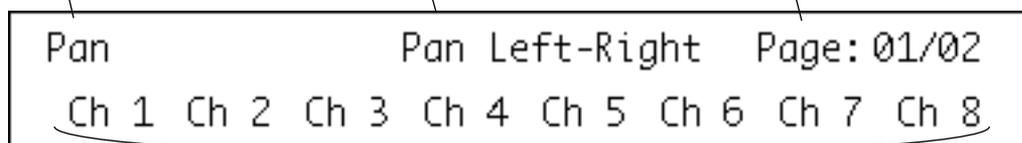
The lower row shows the names of the eight channels in the current Fader Set. You can control the selected parameter for each one of the eight channels by using the corresponding V-Pot. In this example, V-Pot 1 would control the Pan parameter for the channel “Ch1”, V-Pot 2 would control the same parameter for the channel “Ch2” and so on.
