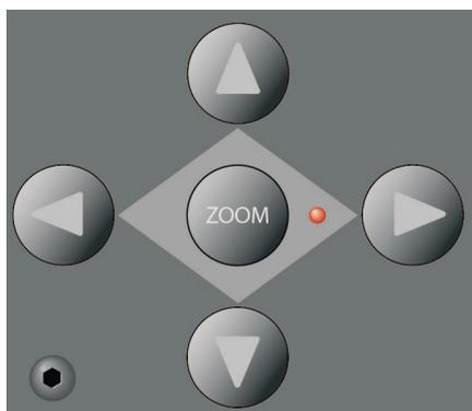
Pressing the cursor keys located to the left of the jog wheel is the same as pressing the arrow keys on your computer keyboard. Note that the Zoom button is not supported.
