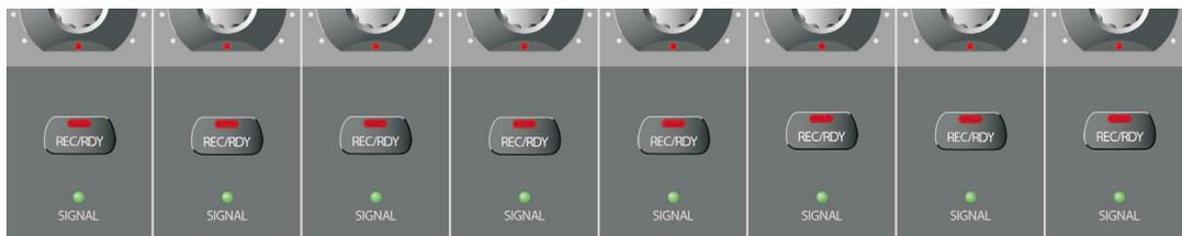
The Signal LEDs underneath the Rec/Rdy buttons indicate signal activity on the channels. The LED lights up as soon as the level meter for a channel shows any activity.
