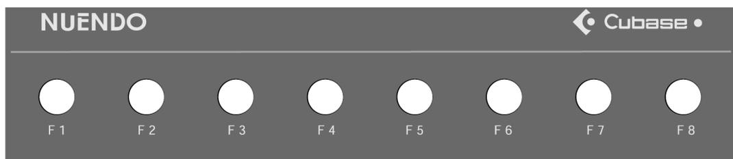
You can use the function keys F1 to F8 and function key combinations with the Shift button to access functions in Nuendo. Refer to the Nuendo operation manual for information about how to assign program functions to remote controller function keys.
