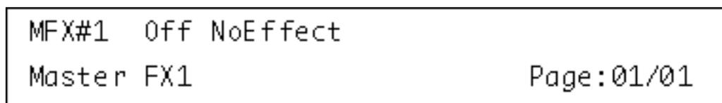
After a plug-in has been selected in Nuendo, the display will change to show the currently selected plug-in this effect slot and the 'number of pages' indicator will be updated to show the amount of pages necessary to display all the plug-in's declared parameters.
